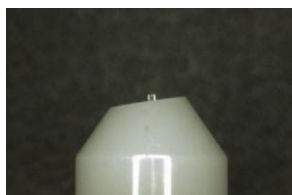
Pre-angled ferrule's end-face with fiber protruded
